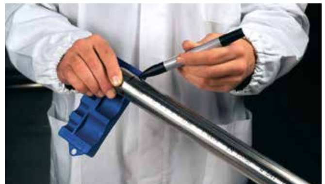
Figure 8 - Marking the insertion depth
