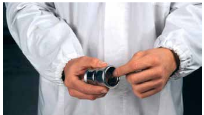
Figure 9 - Checking the sealing ring
