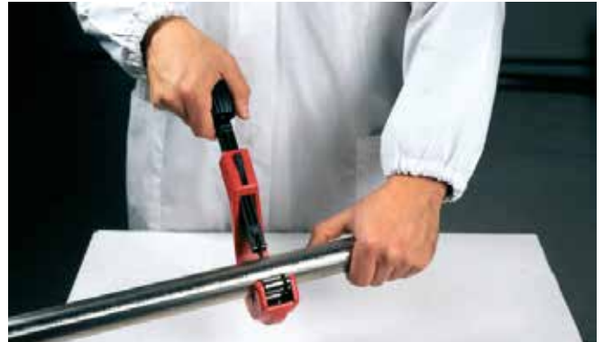
Figure 5 - Cutting the pipe to length
